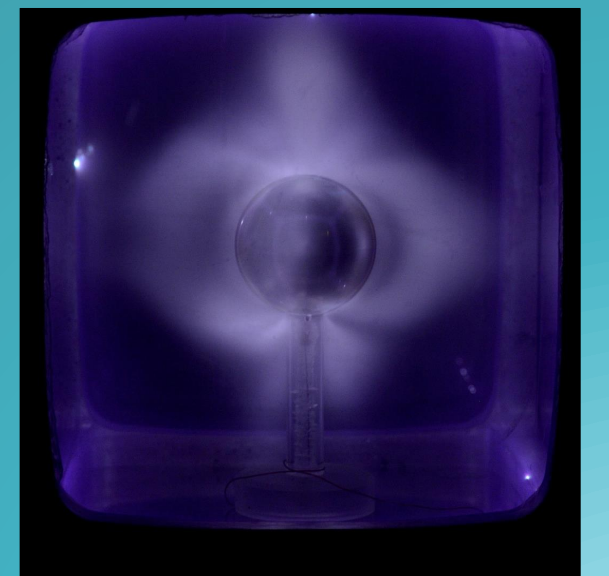
Figure 4. Terrella Cubica in it's • (top) Ring current mode; cathode: the aluminium ball with a magnet • (bottom) Aurora mode; cathode: the aluminium frame
