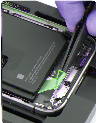
iPhone batteries are secured using advanced adhesives that are designed to release when stretched in a specific direction, enabling battery replacement.
