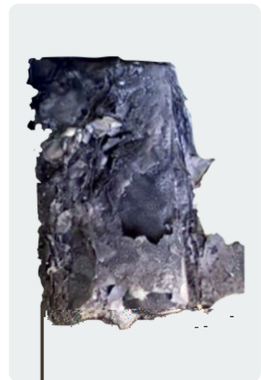
Third-party battery after an Abusive Overcharge test, which is intended to simulate charging the battery beyond its intended limits.
