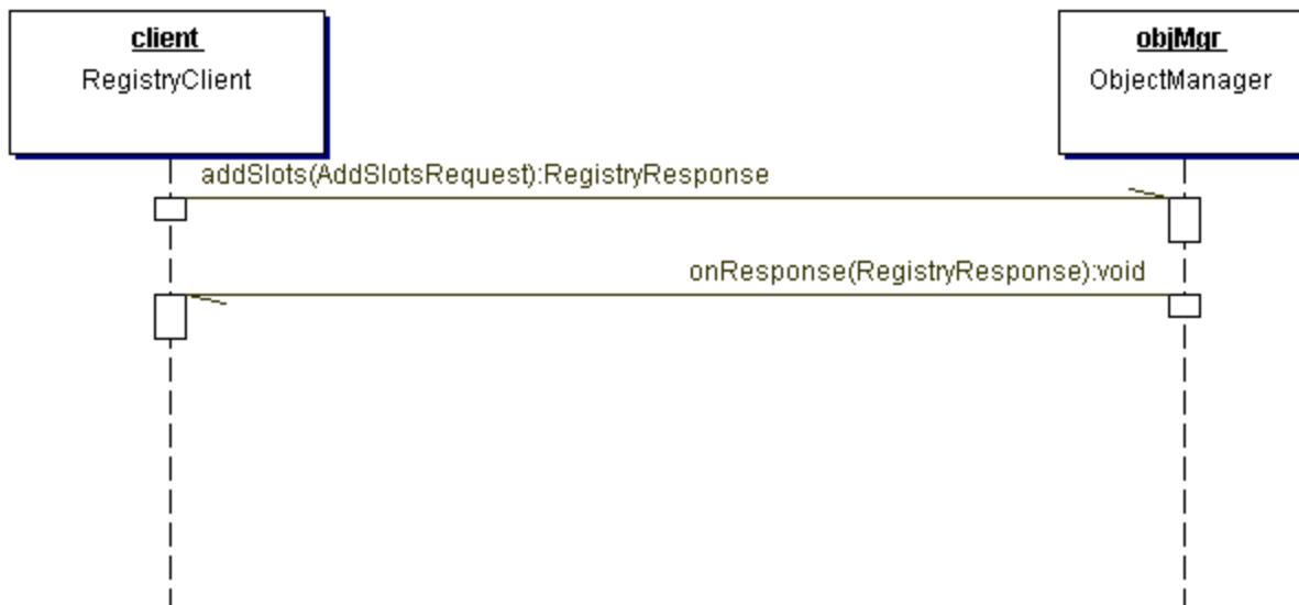
721 722 Figure 7: Add Slots Sequence Diagram
