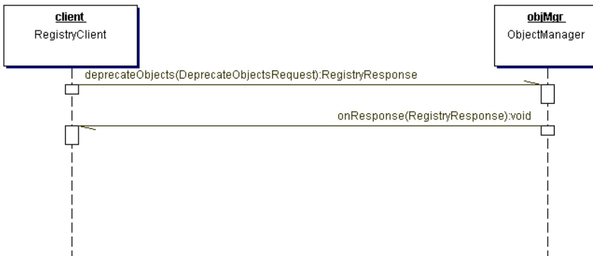
Figure 10: Deprecate Objects Sequence Diagram
