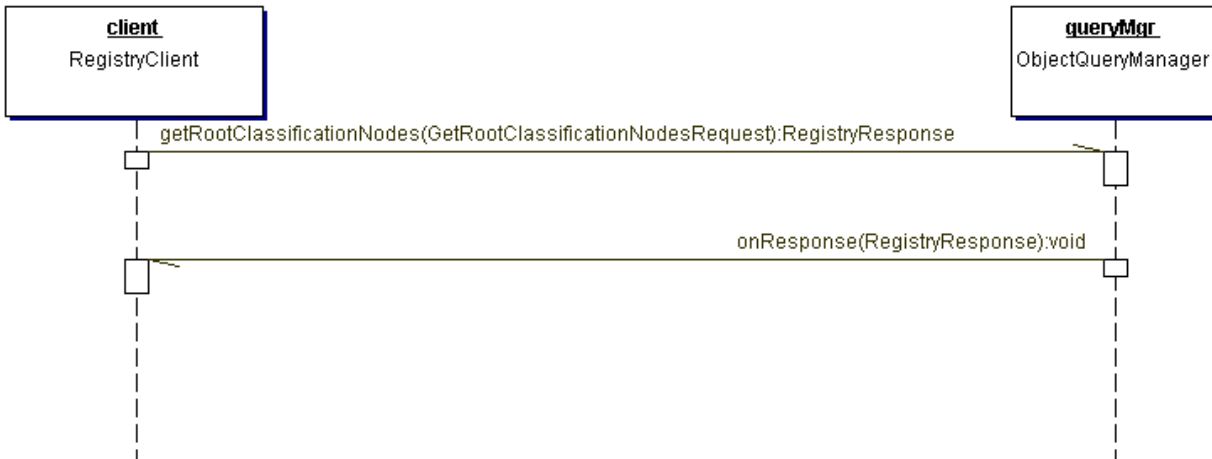
Figure 12: Get Root Classification Nodes Sequence Diagram
