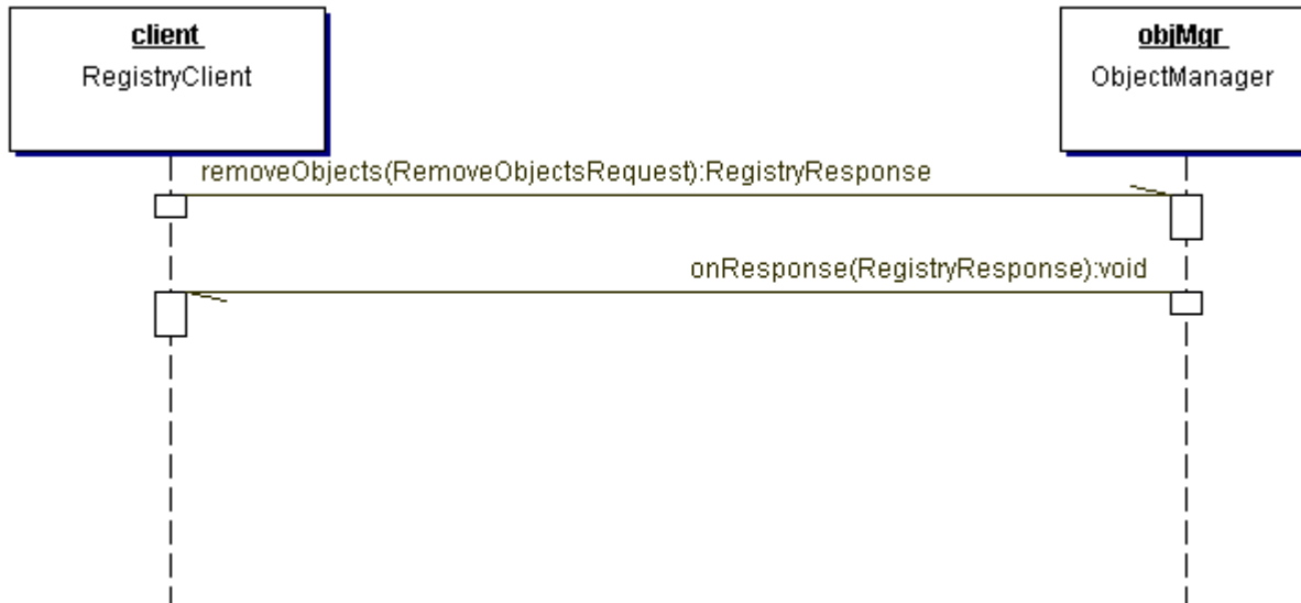
Figure 11: Remove Objects Sequence Diagram
