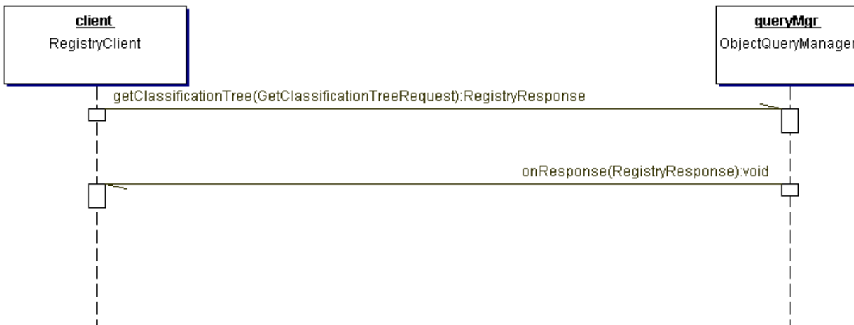
Figure 14: Get Classification Tree Sequence Diagram
