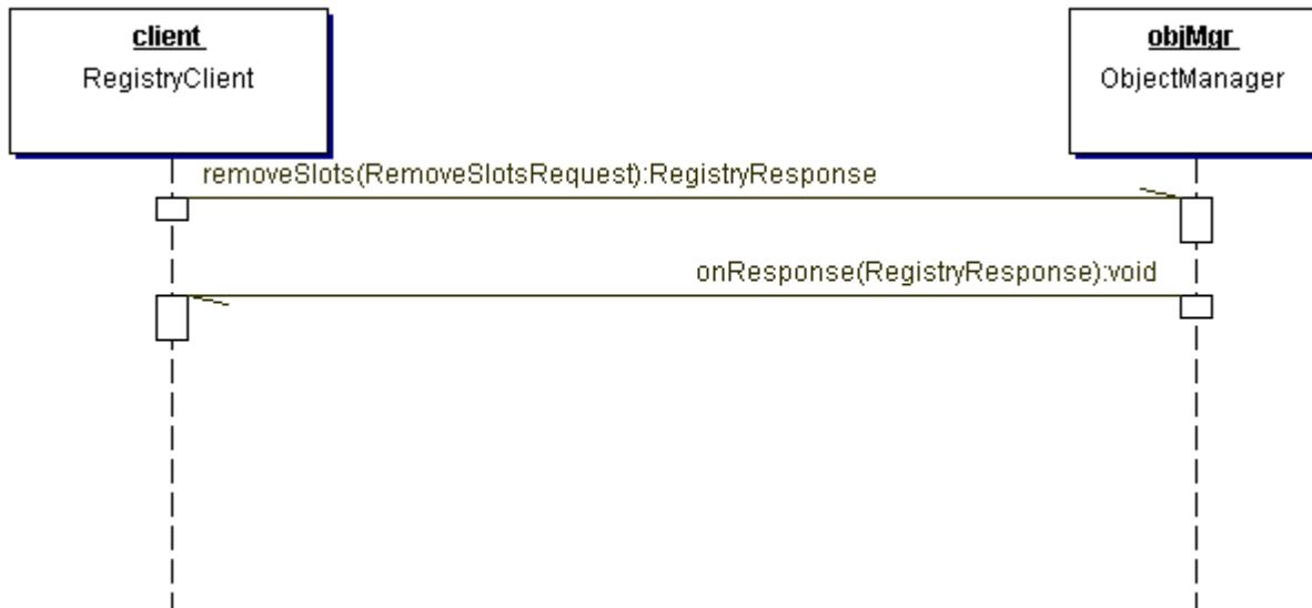
Figure 8: Remove Slots Sequence Diagram
