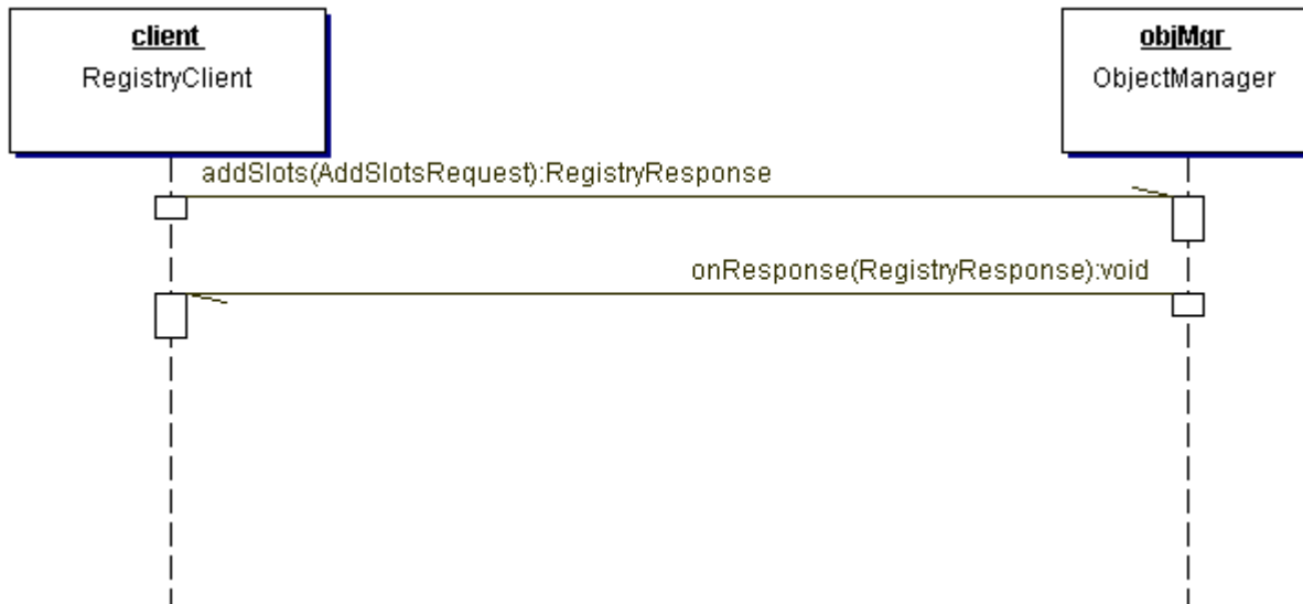
Figure 7: Add Slots Sequence Diagram
