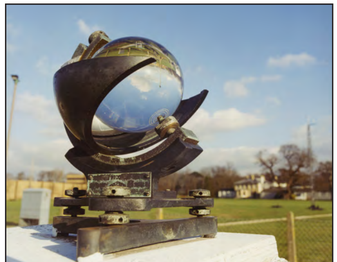
Left: Sunshine cards – different shapes are used during winter, spring/autumn and summer. Right: A Campbell-Stokes sunshine recorder.
