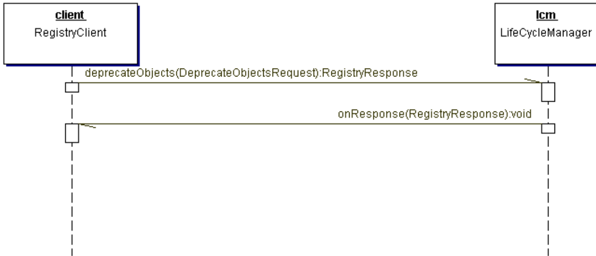
Figure 12: Deprecate Objects Sequence Diagram
