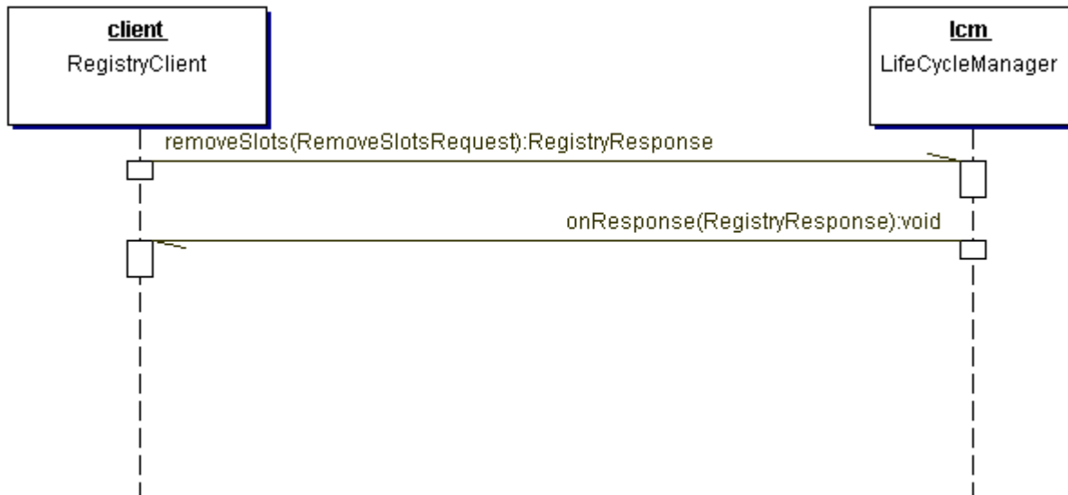
Figure 10: Remove Slots Sequence Diagram
