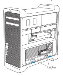
3 Pull the latches until they open all the way and release the processor tray.
