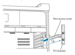
3 Remove the port access cover from the slot in which you plan to install the card.
