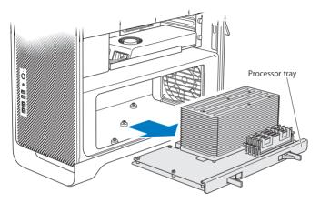
If you install equal-size DIMMs (for example, all 1 GB DIMMS or all 2 GB DIMMS) in your quad-core or 6-core Mac Pro, Apple recommends that you fill the slots in the order listed in the table.
