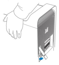
You can attach a lock or cable through a metal loop (under the latch) to secure your Mac Pro. Flip the metal loop down before you close the latch, then close the latch and attach your lock or cable through the extended loop.
