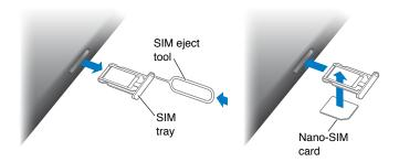
Open the SIM tray. Insert a SIM eject tool into the hole on the SIM tray, then press firmly and push the tool straight in until the tray pops out. Pull out the SIM tray to install or replace the SIM card. If you don't have a SIM eject tool, try the end of a small paper clip.
