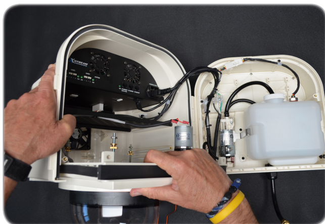
Figure 8.3 - Removing the camera tray.
