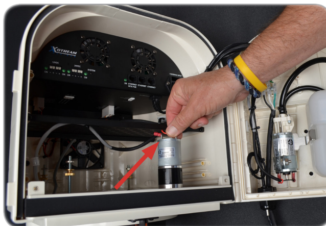
Figure 8.2 - Disconnecting the motor cables.
