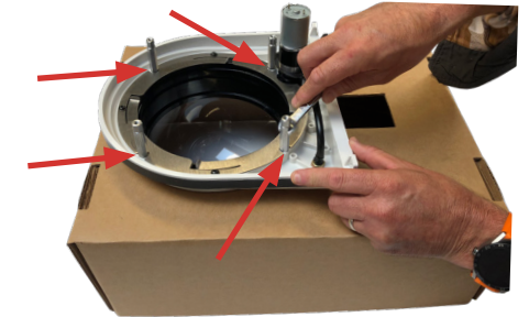
Figure 12 - Securing the standoffs into the lower tray assembly.
