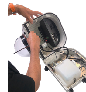
Figure 3 - Removing the lower tray assembly.
