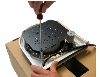
Figure 14 - Securing camera mount assembly to the standoffs.
