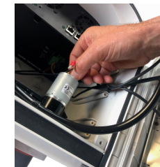
Figure 2 - Disconnecting Power Leads
