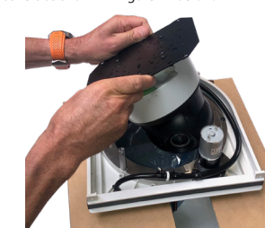
Figure 13 - Lowering camera assembly onto the standoffs.
