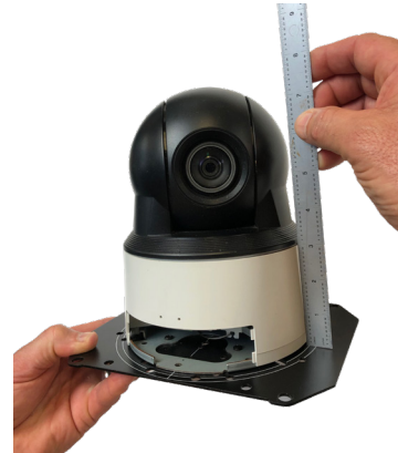
Figure 9 - Measuring the height of camera assembly.
