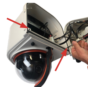
Figure 1 - Removing lower tray fastening screws.
