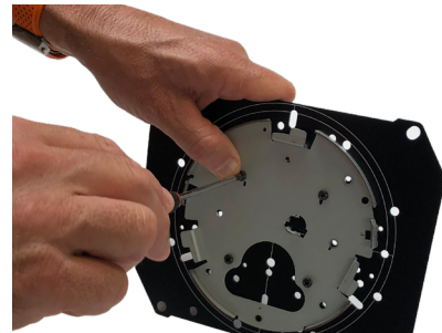
Figure 8 - Attaching camera mounting hardware.
