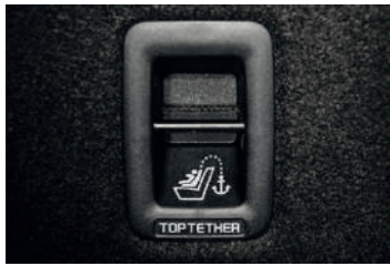
ISO Child Anchor: Keep your child safely and securely seated by strapping their seat to the special metal anchors in the vehicle.
