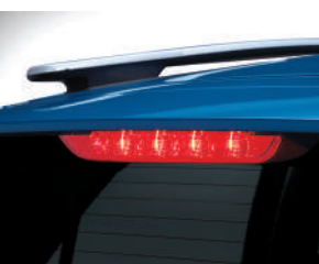
High Mounted Stop Lamp (HMSL): The high mounted stop lamp integrated in the rear spoiler, let other vehicles vividly see you stopping on the road.
