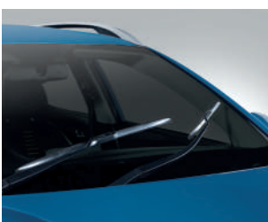
Aero Blade Wipers: Aerodynamic wiper blades maintain contact with the windshield, even at high speeds.
