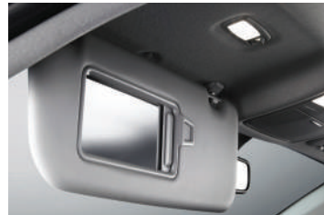
Sun Visor Illumination Lamps: Tasteful LEDs beside the vanity mirror on the driver-side sun visor light up to help with last minute touch-ups.
