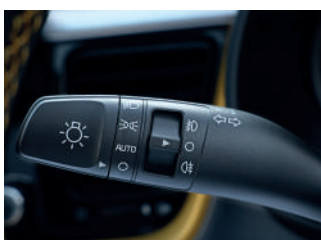
Auto Light Control: The headlamps are engineered to respond smartly to external light and adjust to its levels for better driving facilitation in the night time.
