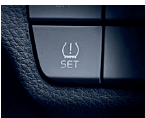
Tire Pressure Monitoring System (TPMS): Tire Pressure Monitoring System (TPMS) in your Stonic is designed to alert you of a change in tire pressure that could put you at risk.
