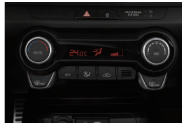
Auto Climate Control: Auto temperature control lets you select a desired temperature for the system to maintain. A digital readout displays temperature and settings.
