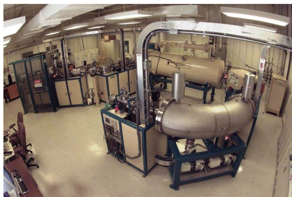
Figure 4 | Measuring ^{14}\text{C} is now most commonly done with an accelerator mass spectrometer. US DOE, public domain
