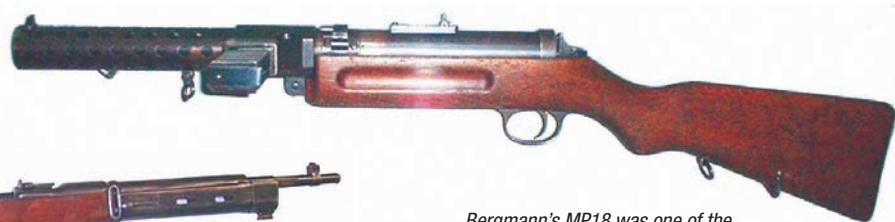
Bergmann's MP18 was one of the first mass production submachine guns, firing 9 mm pistol rounds. A key contributor in the design was Hugo Schmeisser who later designed the MP43.
