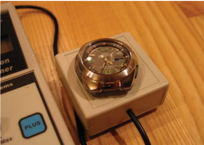
5. Measuring an analog radio controlled wristwatch between synchronizations.
