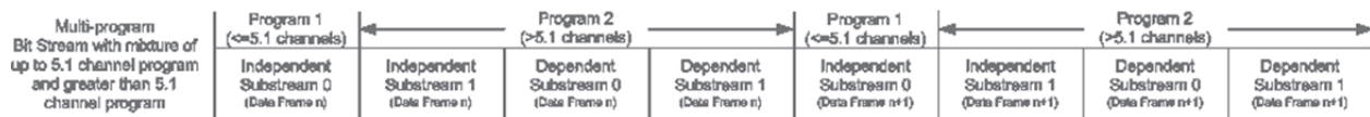
Figure E3.5 Bitstream with mixture of programs of up to 5.1 channels and programs of greater than 5.1 channels.
