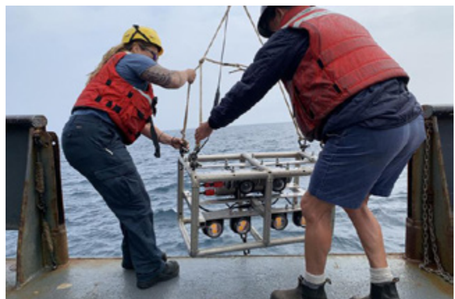
Deploying the stereo camera system over the starboard side of the Canadian Coast Guard vessel John P. Tully . Credit: NOAA Fisheries/Paul Hillman
