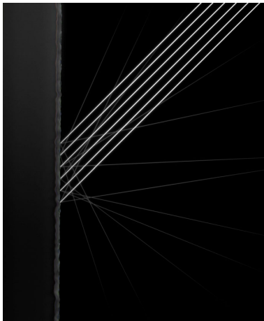
Light scattering on nano-texture cover glass
