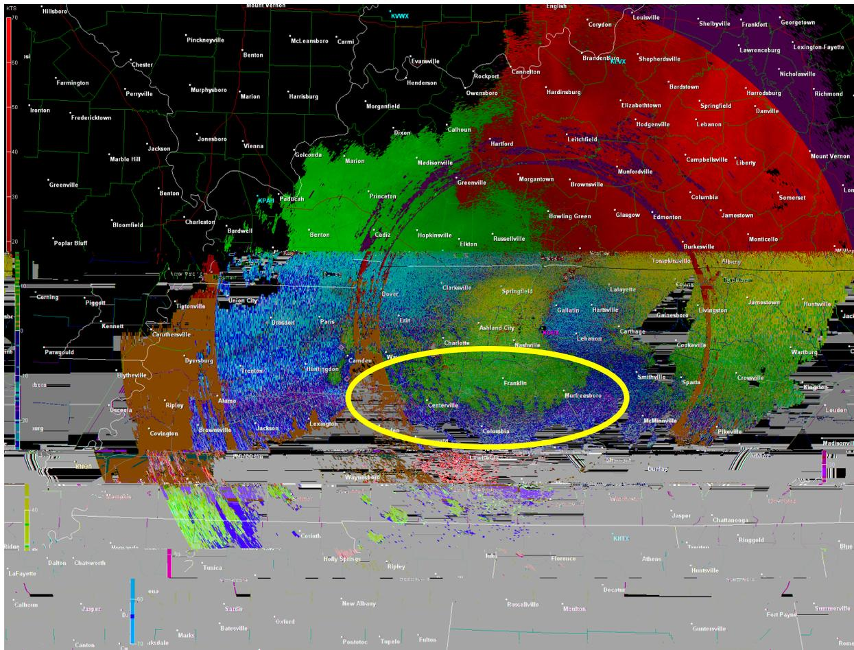
*Figure 12: Base velocity image from KOHX (Nashville, TN) for 16 UTC on 1 May, 2010. Yellow outline denotes the mesoscale boundary that remained stationary through most the day, serving as a constant focus for the development of new convection.*
