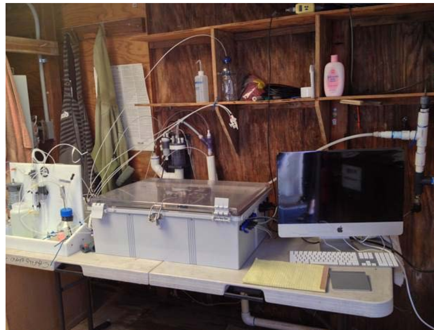
The “Burk-o-lator” – developing low cost OA sensors
