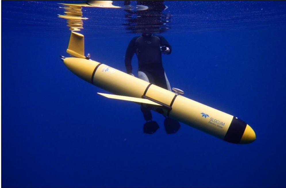
Figure 1. Slocum glider (photo courtesy of Rutgers University).
