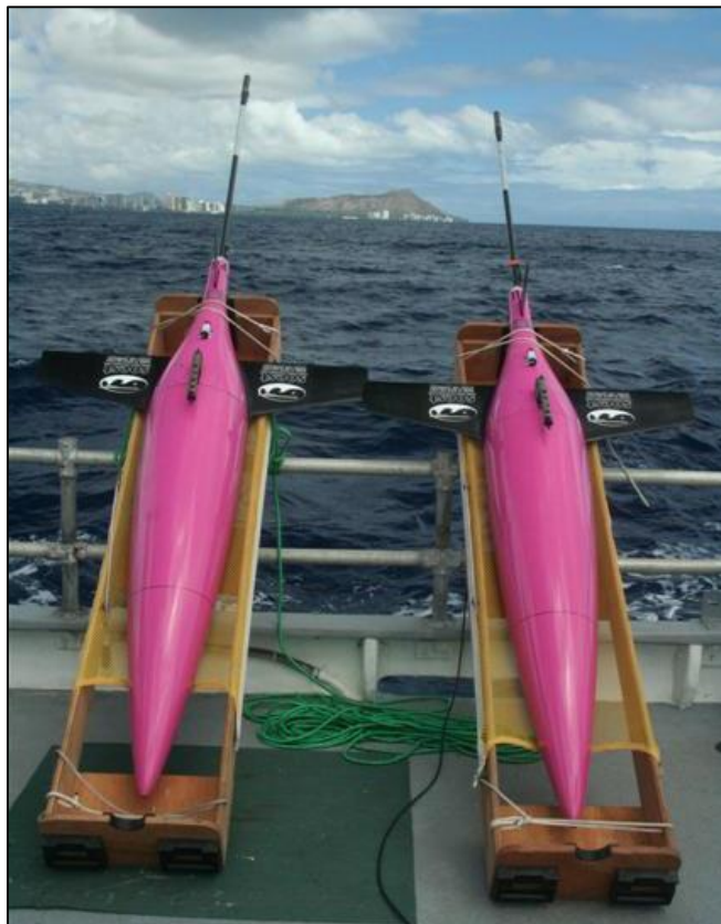
Figure 2. Seaglider (photo courtesy of the School of Ocean and Earth Science and Technology at the University of Hawaii at Manoa).
