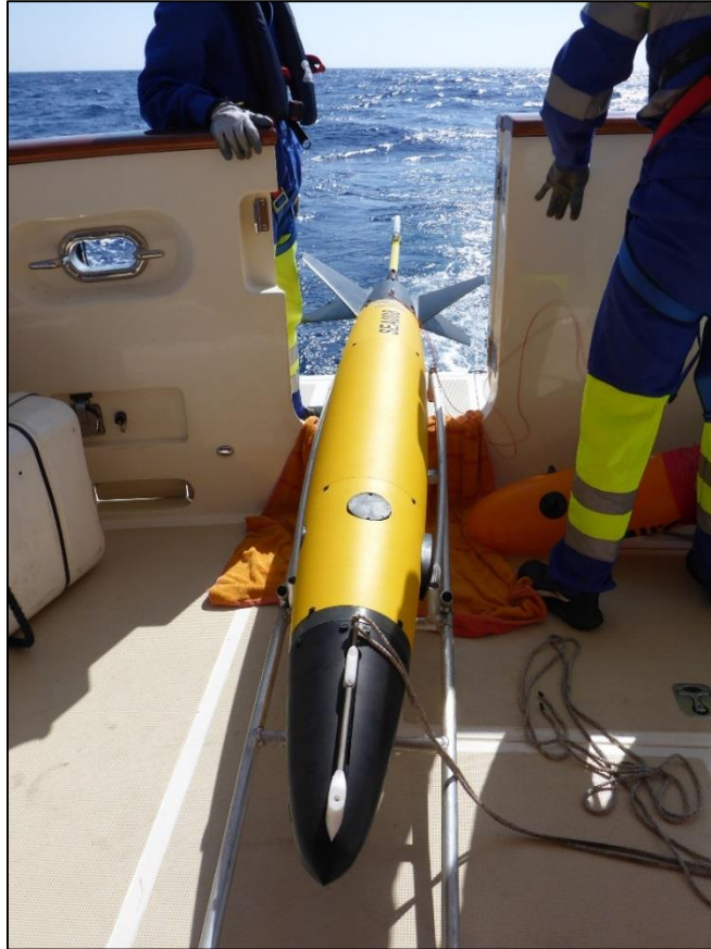
Figure 3. ALSEAMAR Sea Explorer (photo courtesy of Romain Tricarico/ALSEAMAR and Stephanie Jaeger/Sea-Bird Electronics).
