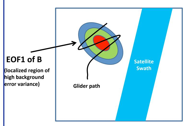
The glider path does directly observe the region of high error background error variance associated with EOF1 of B, so errors in this regions will be corrected during data assimilation by the glider.
