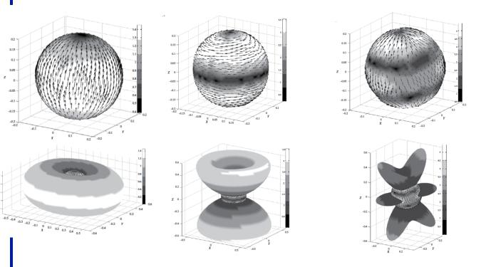
Examples the induced currents and electric and magnetic fields associated a selection of the leading eigenmodes of the impedance matrix of a perfectly conducting sphere (adapted from Chen and Wang, 2015).
