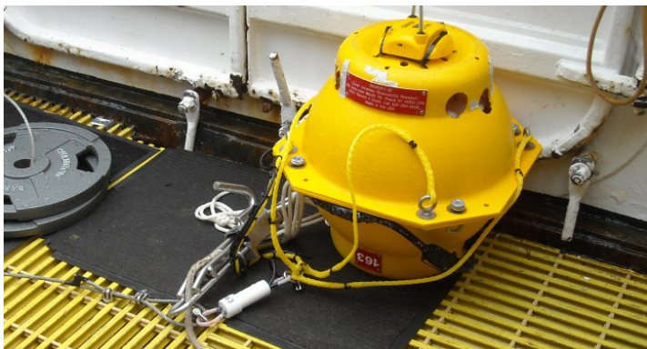
A Marine Autonomous Recording Unit (MARU) used by scientists at NOAA's Northeast Fisheries Science Center to record sound on the ocean floor.
