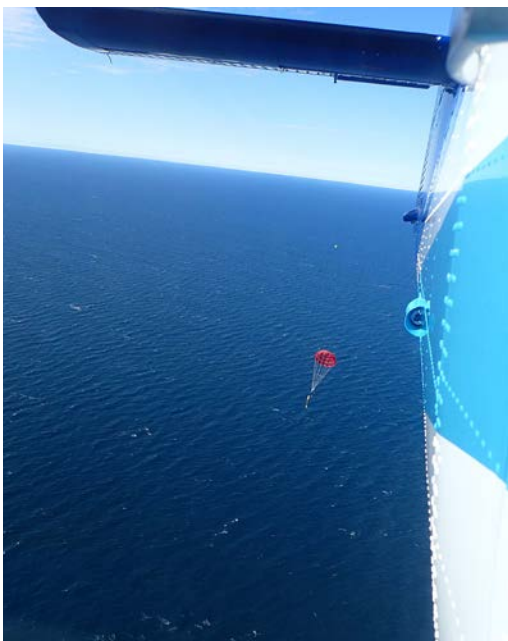
An Air-Launched Autonomous Micro-Observer (ALAMO) float is deployed from NOAA's Twin Otter allowing NOAA's Pacific Marine Environmental Laboratory and Climate Program Office to study sea ice.
