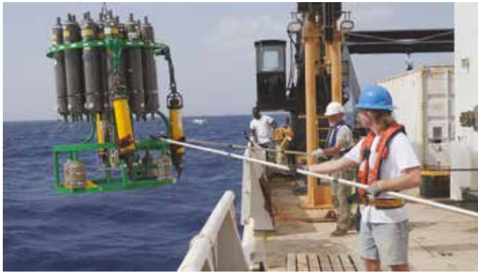
Scientists lower Conductivity, Temperature, Depth Rosette into the Atlantic Ocean off Barbados. Credit: Richard Marchbanks/CIRES NOAA (January 2020)
