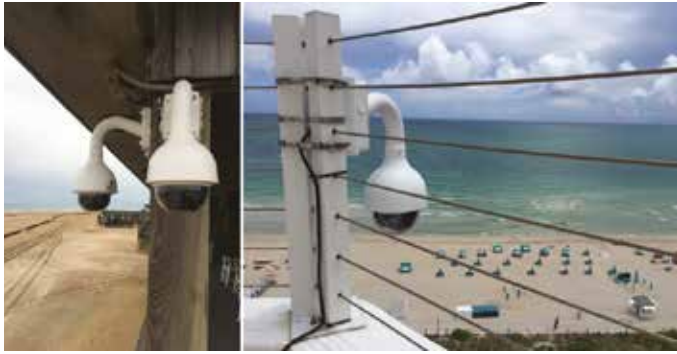
The Buxton, NC (left) and Miami Beach, FL (right) webcams installed as part of the pilot webcam observation network. Image Credit: Surfline Inc.
