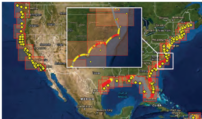
The Nearshore Wave Prediction System coverage for the continental U.S., with an inset box showing hazardous rip current likelihood for the North Carolina coast. Alongshore color denotes rip current likelihood from low (gray) to high (red). Image credit: NOAA
