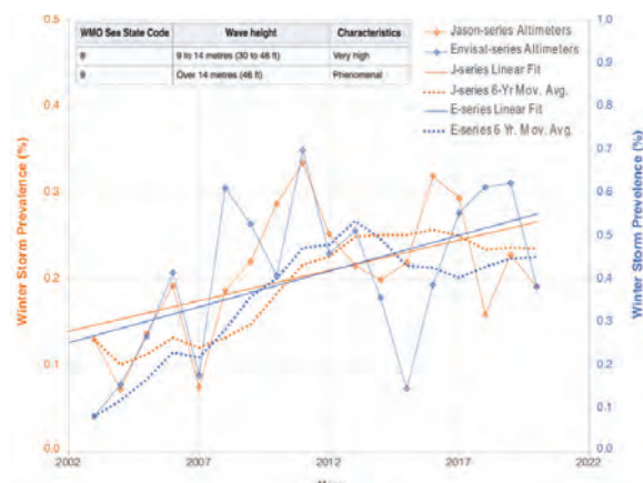
Trends in very high and phenomenal sea state in the Bering Sea in winter. Two independent measurements show an increase in storminess in the Bering Sea over the last 16 years. Graphic credit: Sinead Louise Farrell, Kyle Duncan and John M. Kuhn, "Altimetry of the Arctic Ocean and Subpolar Seas Ocean Surface Topography Science Team Report: 2016-2020"
