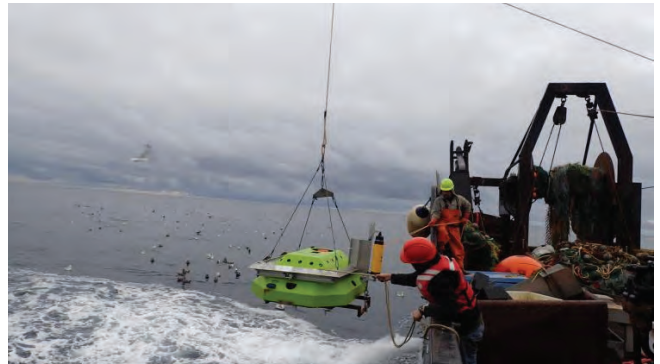
Deploying the echosounder to monitor pollock movements in the Bering Sea. Photo credit: Leah Zacher, NOAA Fisheries
