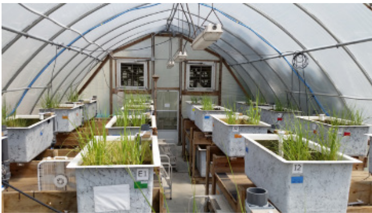
NOAA salt marsh mesocosms in Charleston, SC used for testing recovery of oiled marshes. Image Credit: NOAA
