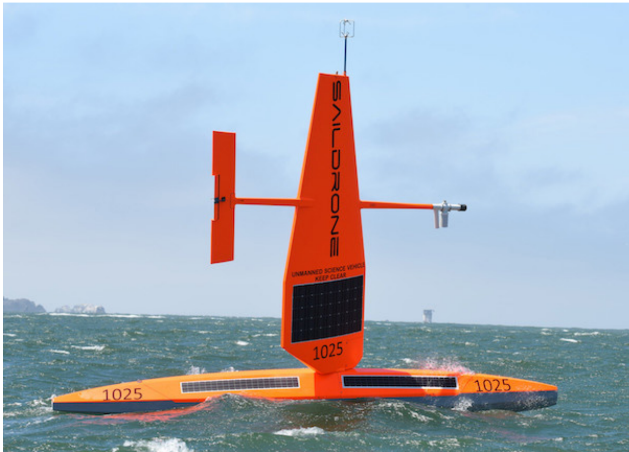
A saildrone maneuvering by wind. Note the solar panels that are used to power the onboard instruments. Photo credit: Saildrone, Inc.
