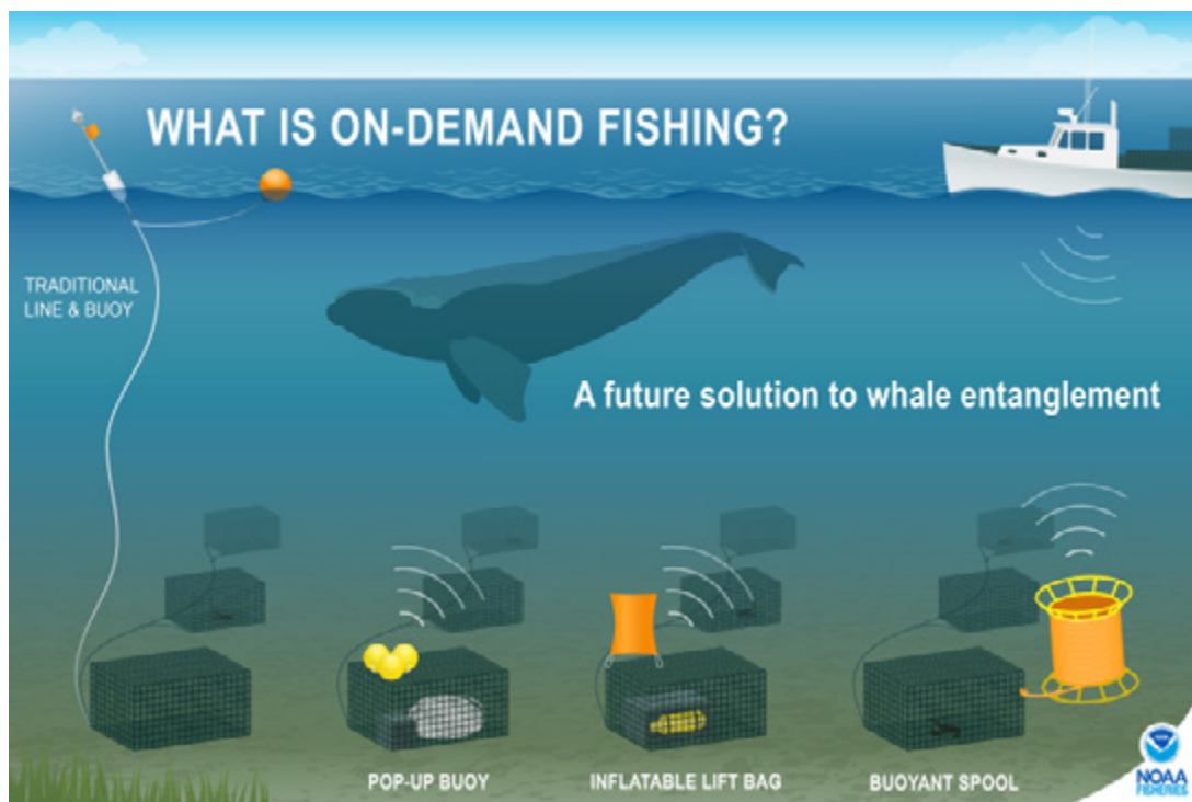
On-demand, also called “ropeless”, systems use far less rope in the water than traditional gear designs. To locate and retrieve gear, traditional methods tether gear to a rope attached to a buoy at the water’s surface. The main characteristic of on-demand gear is that it does not need this gear-to-buoy tether. Credit: NOAA Fisheries
