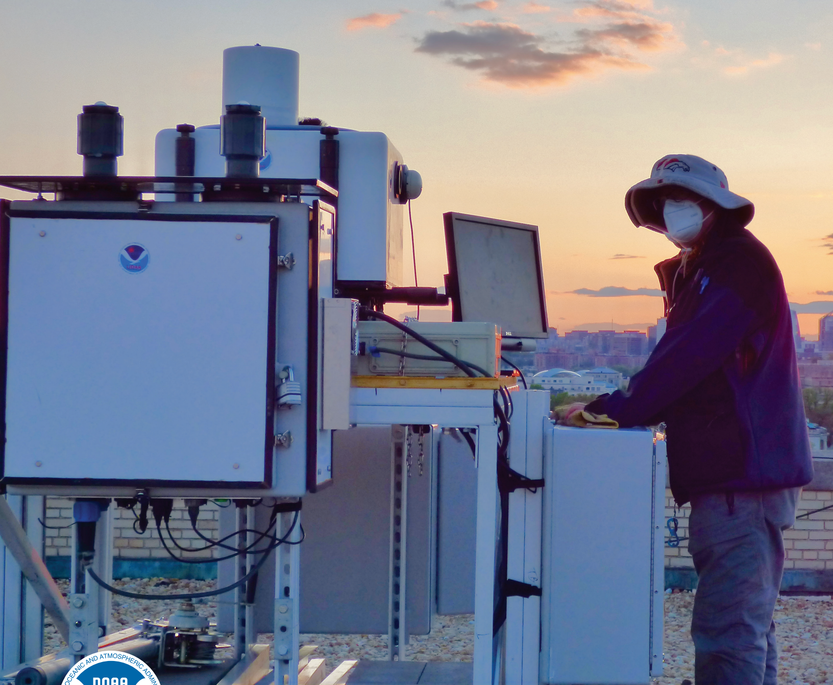
Scott Sandberg, an electrical engineer with NOAA's Chemical Sciences Laboratory, worked with Tyler Boyle of NIST to install a Doppler lidar instrument on April 16, 2021, on top of the Department of Commerce's Herbert Clark Hoover Building in Washington, D.C. for a research project studying urban greenhouse gas emissions. Credit NOAA's Scott Sandberg and NIST's Tyler Boyle
