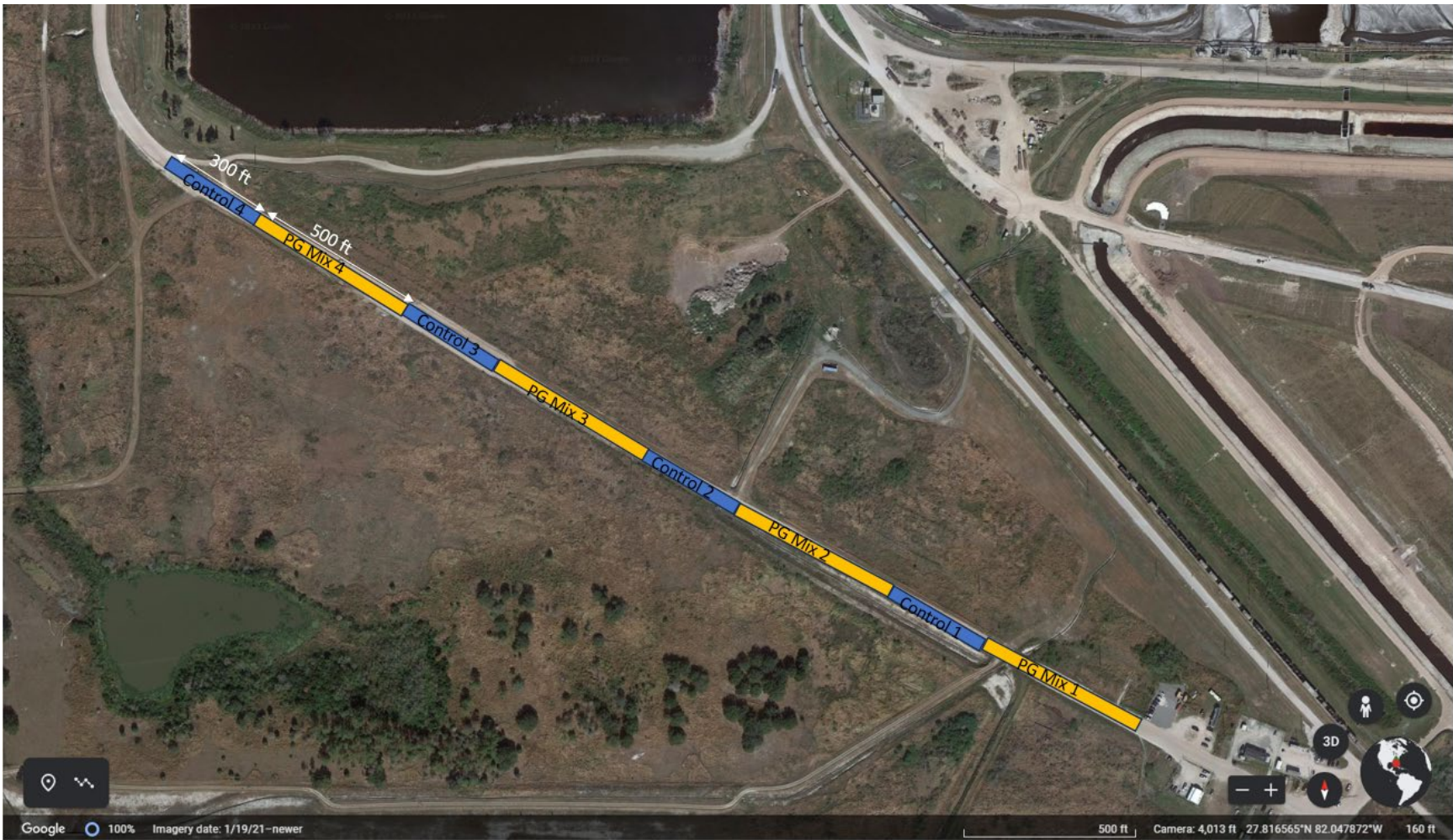
Figure 2-2: Pilot road configuration. The road will be 3,200 ft long with alternating segments of 500-ft PG-mix designs and 300-ft controls (no PG added).
