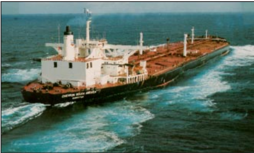
The Chevron South America received a 1999 outstanding VOS performance award from Norfolk PMO Pete Gibino. She is one of the 15 largest vessels in the world, at 1200 feet long with a beam of 229 feet. The vessel can carry 3,162,635 barrels of oil (about 407,000 tons) at 98% full. Draft at full load is 75 feet. With a 42,000 HP steam engine, she has a service speed of about 15.3 knots loaded and 17 knots in ballast.
