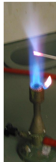
Figure 3 | Flame test: lead colors flame pale blue Herge, public domain
