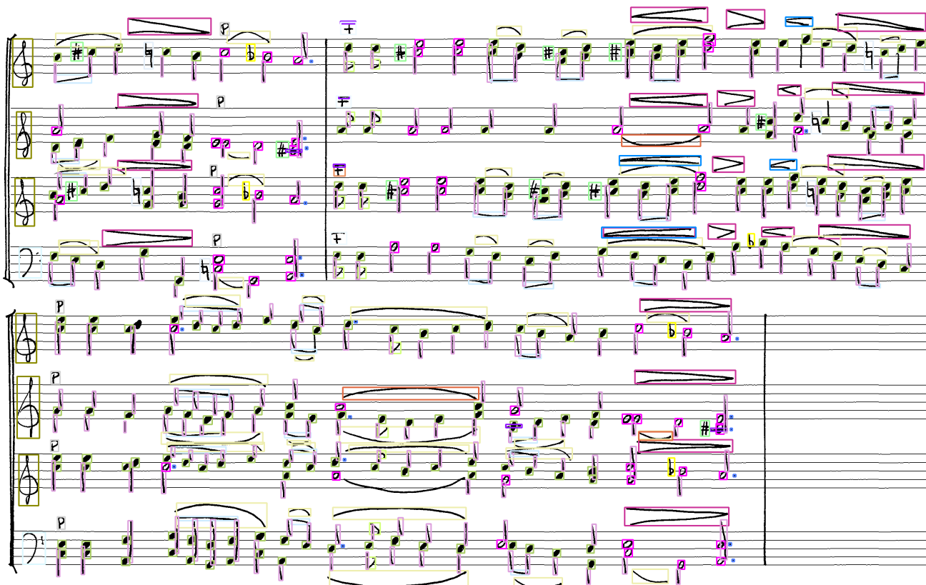
Figure 3: Sample output of the improved music object detector. Each detected object v has a box around it, with the color representing the class \zeta(v) of the particular object, e.g., light green for full-noteheads.
