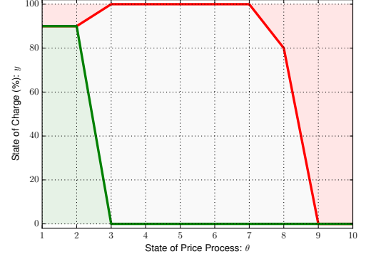
Figure 3: Example of a threshold policy. The upper (red) line represents C(\theta) ; the lower (green) line represents c(\theta) .
