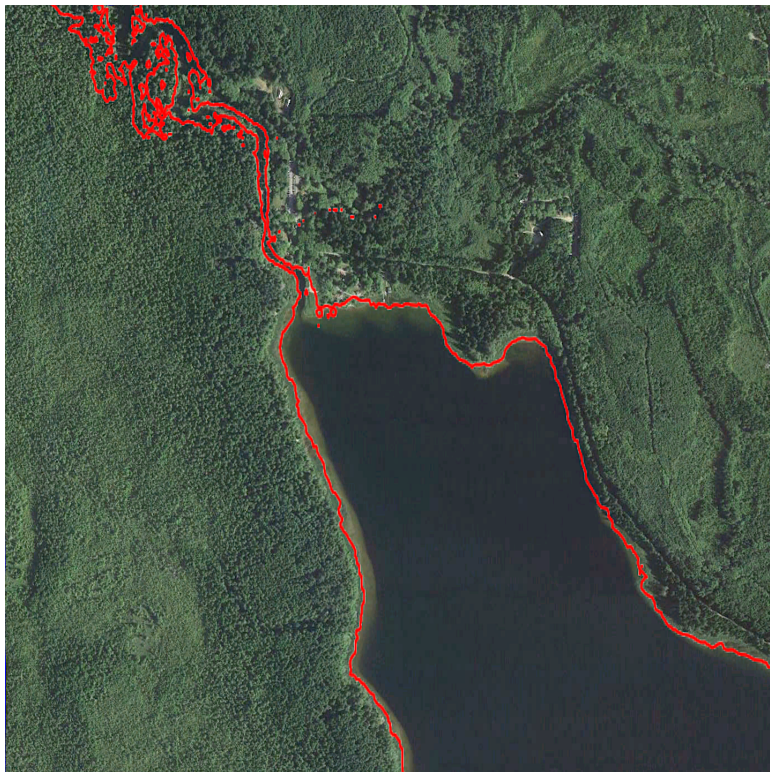
Figure 14: Top: Zoomed view of Figure 13 showing the north shore and the outlet into the Ozette River. The red contour at 9.2 m shows the approximate shoreline. This elevation was chosen as approximately the minimum elevation that gives a connected river at the saddle point. In this plot the blue contours are at 0, -2, -4, ..., -18 m and green contours at +2, +4, ..., +18 m relative to MHW. Moreover, here the blue background fills out to the red contour (the presumed lake shoreline), for better comparison with the bottom figure, which shows imagery of the same region from Google Earth together with the 9.2 m contour.
