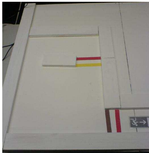
Fig. 8. An example toy world labyrinth in which we tested the one-way road pledge. The marks on the floor represent the one-way roads. A red color indicates the side from which the robot may not pass. Other colors are used to identify each one-way road and the side, from which the robot may pass.
