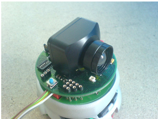
Fig. 7. The Khepera II with a CMUCam turret. The wires are only used to submit status messages. The whole computation is done on the Khepera itself.
