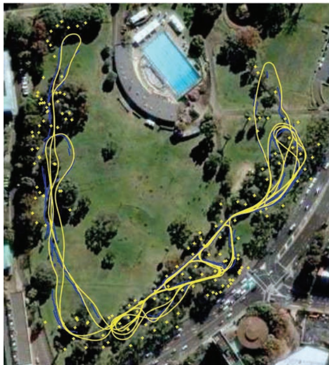
Figure 6: Optimized map of the full Victoria Park sequence. Solving the complete problem after every step takes less than 2 minutes on a laptop for known correspondences. The trajectory and landmarks are shown in yellow (light), manually overlayed on an aerial image for reference. Differential GPS was not used in obtaining the results, but is shown in blue (dark) where available. Note that in many places GPS is not available.
