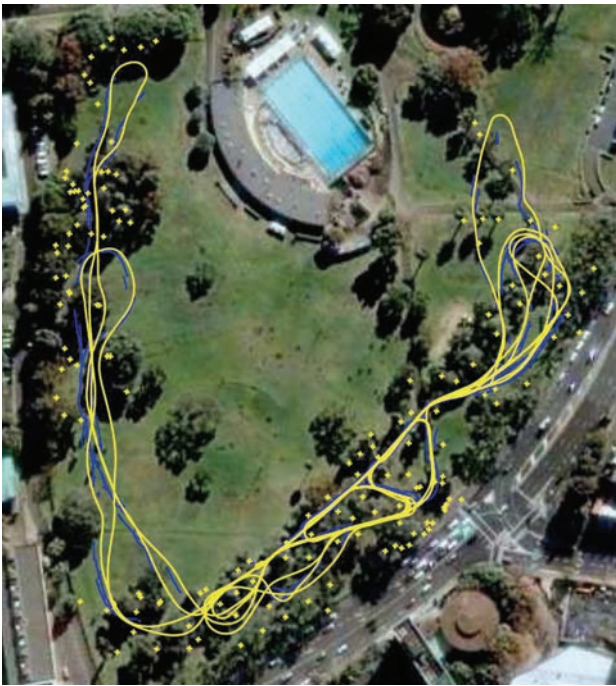
Figure 5: Trajectory and map computed from the Victoria Park dataset overlaid on satellite imagery of the park.
