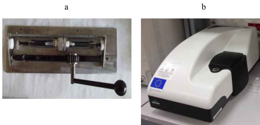
Fig. 1. a) Extruder used for the size calibration, b) ZetaSizer Nano ZS90.
