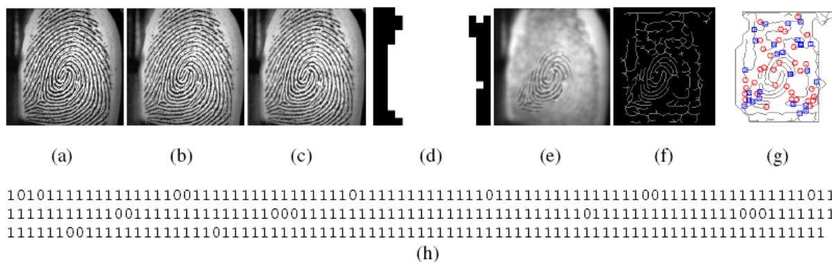
Figure 9: (a) Input Fingerprint Image (b) Histogram Equalized Image (c) Median Filtered Image (d) Segmented Image (e) Enhanced Image (f) Morphological Processed Image (g) Fingerprint images with Minutiae Points (h) Generated irrevocable key.
