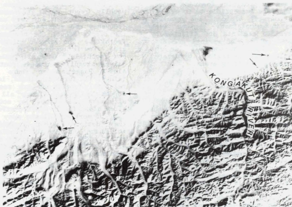
Figure 3. Winter Landsat image (band 7) of the Demarcation Bay area. Stream overflows (B) are dark and coincide with ice sheets displayed in Figure 2. Several unlabeled overflows are present.
