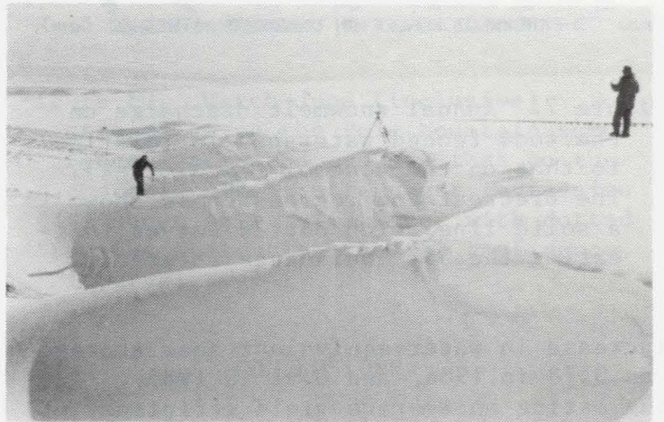
Figure 6. Snowdrift on the lee side of the fence at time of peak accumulation in 1985. The top of the streamgage instrument shelter is visible in the background.
