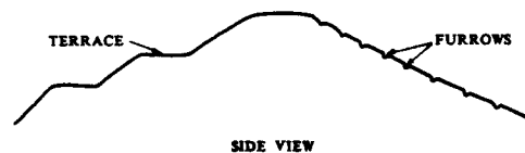
Figure 5. Terraces and furrows on side slopes.
