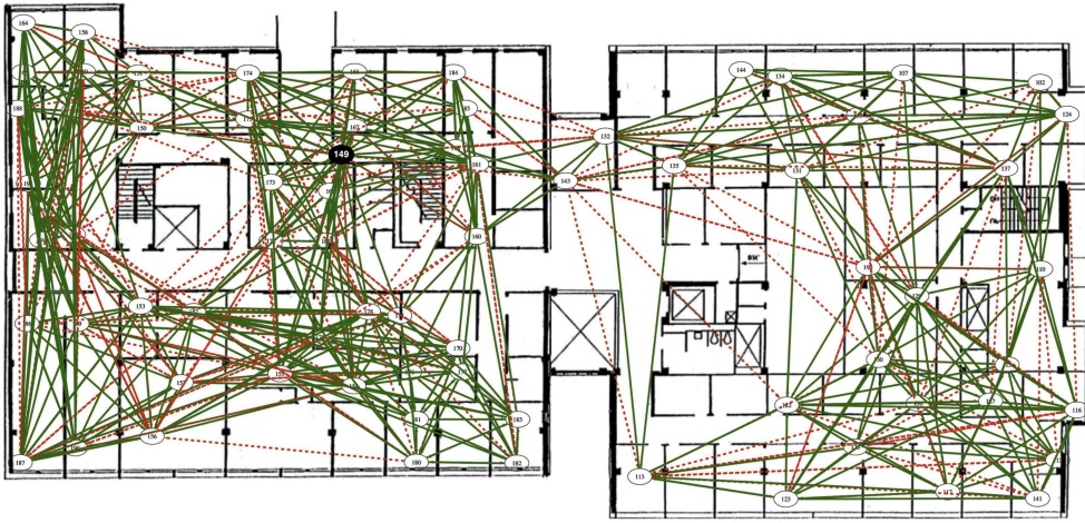
Fig. 11. Testbed topology at -5 dBm Tx power (solid green lines are communication link; dotted red lines are interference link; the solid black node is the sink)
