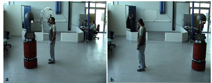
Fig. 15. Visibility criterion effect when passing in front or behind of a human.
