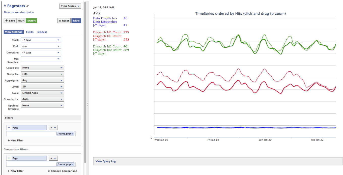
Figure 1: Scuba’s web user interface. The query shown on the left side generates a time series graph with a week over week comparison of three columns related to Facebook page dispatches. The dotted lines represent the same days one week earlier. It is very easy to see daily and weekly cyclical behavior with these graphs.
