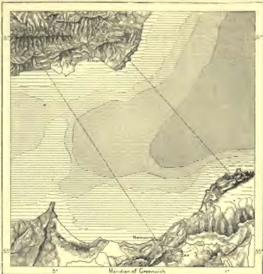
Fig. 66. — JUNCTION OF THE GEODETIC LINES BETWEEN ALGERIA AND SPAIN.
