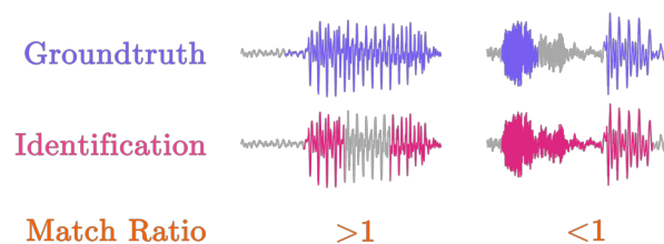
Figure 3. Proposed metric Match ratio. It defines the ratio between the number of identifications with respect to the number of annotations in the groundtruth.
