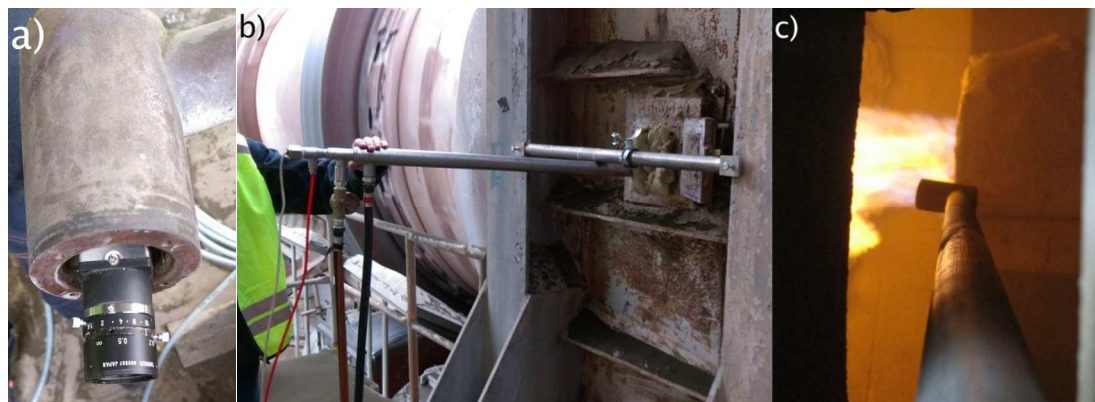
Figure 1: a) The camera inserted in the probe. b) Camera probe inserted through side of kiln hood. c) Camera probe inserted next to kiln burner.
