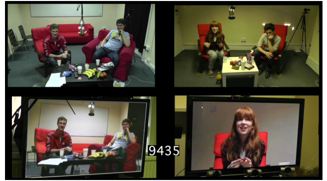
Figure 1: Evaluation setup for social video communication with four people in two rooms that are equipped with one screen and three physical HD cameras each. The Virtual Director decides which video streams to render on screen depending on the communication situation.
