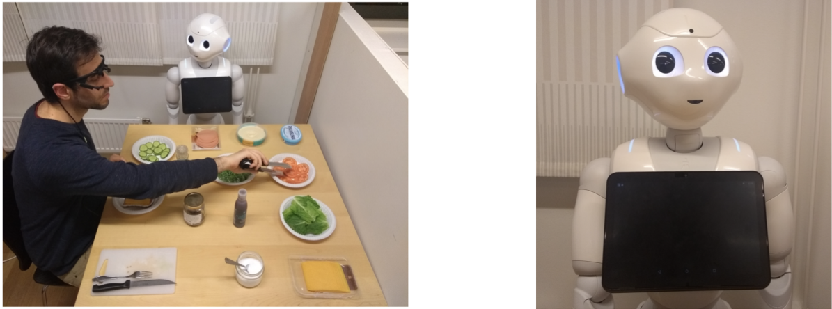
Figure 1: On the left, a picture of the experimental setup during an interaction. The participant takes an ingredient following the instructions of the agent. On the right, the Pepper robot used for this study.
