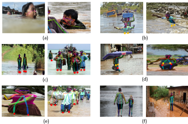
Figure 2: All cases of the result predicted by OpenPose (Red/yellow circle illustrates the knee/hip keypoint meet the conditions of each case). (a) Swimming person with pose from the neck upward, (b) Hip keypoint outside of the person, (c) Knee keypoint outside of the person, (d) Keypoint fit with the person but the ratio of thighs is very small compared to the upper body, (e) Knee keypoint close to the submerged part, (f) Normal pose of the person not submerged
