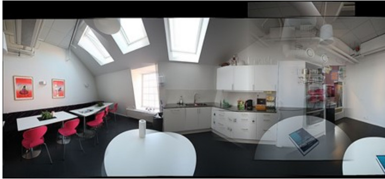
Figure 8: Panoramic image obtained from 6 frames of the "LunchRoomBlue" image set with an angular displacement of 45 degrees between frames using the OpenCV algorithm (ORB).
