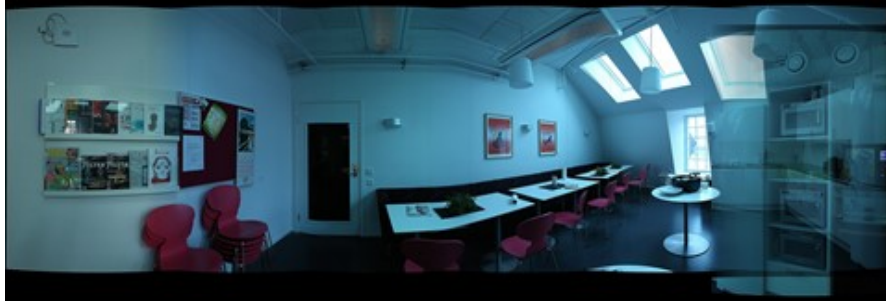
Figure 5: Panoramic image obtained from 8 frames of the "LunchRoomBlue" image set with an angular offset of 35 degrees between frames using the OpenCV algorithm (ORB).
