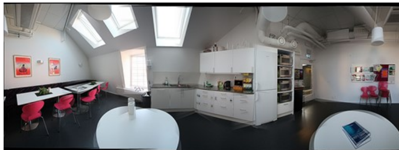
Figure 7: Panoramic image obtained from 6 frames of the "LunchRoomBlue" image set with an angular displacement of 45 degrees between frames using the OpenCV algorithm (SURF).
