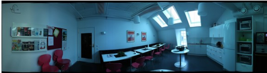
Figure 3: Panoramic image obtained from 8 frames of the "LunchRoomBlue" image set with an angular displacement of 35 degrees between frames using the developed algorithm.
