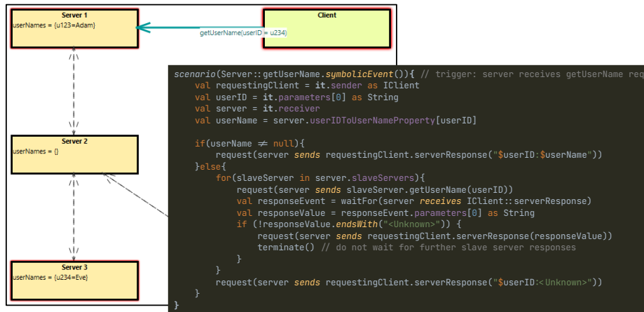
Fig. 2. An example SMLK scenario of a simple hierarchical name lookup system with interaction animator UI screenshot
